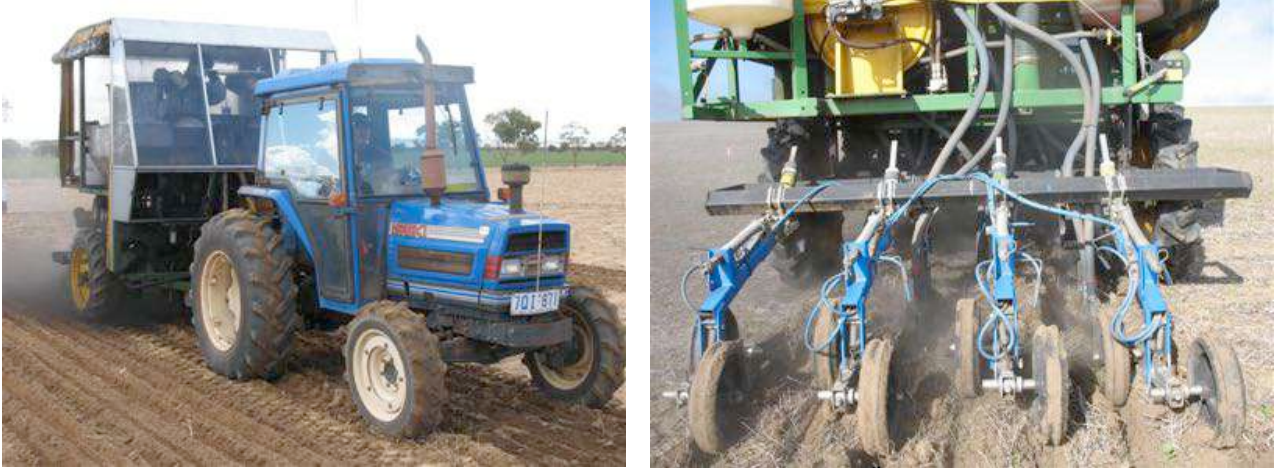
Figure 3. Banding of biochar using a coneseder at Kalannie on 18 th June 2008.
